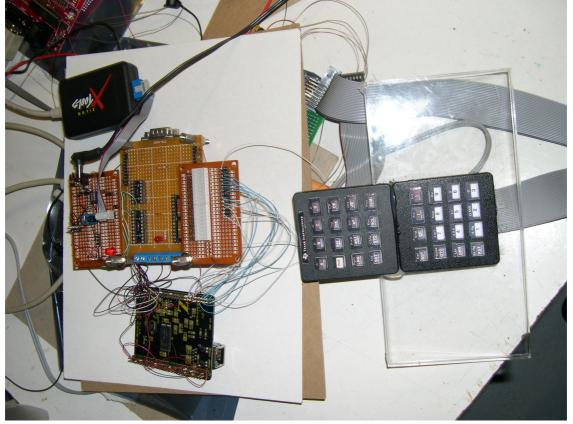
Photo 3b - Shows the prototype TI-59 Programmable Calculator including the custom keypad with TI-59 function key labels glued to each keypad key. Not shown are the thirteen pushbutton switches.
