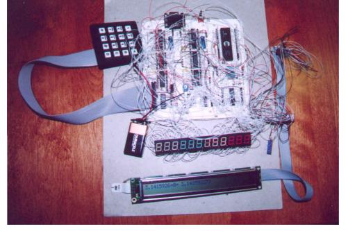
Photo 4 – Is a snapshot of the large 12-digit numeric LED Display Driver Board.
