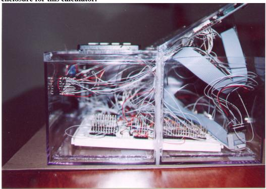
Photo 2b– You can see the wire-wrap construction very clearly using the clear plastic enclosure for this calculator.
