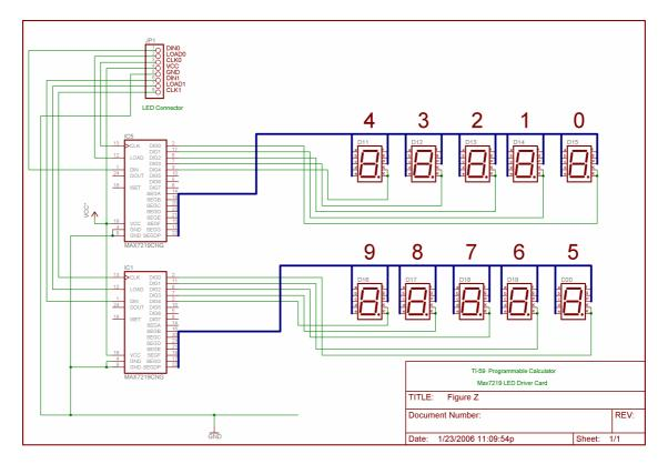
Photo 5 – Shows the MAX7219 LED Display Driver Board.
