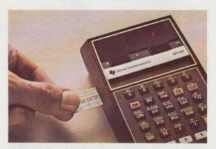
2. Remove card. And send the magnetic card through again. This time the B-side.
