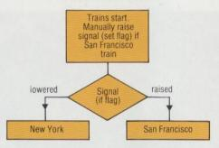
In another situation, the trains themselves can set the signals. Therefore, as dispatcher, you only monitor which tracks are being used. Similarly, on the SR-52, you can have the program automatically set the flag based on data. And the program tests the flag's condition to automatically guide the program to the correct conclusion.
