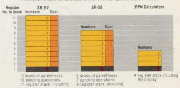
A calculator with full AOS remembers both the numbers and functions in its register stack. And performs them according to algebraic hierarchy. As more operations become pending, the stack fills up (see diagram). Finally, when the equals key is pressed, the operations in the register stack are performed to give you the correct answer (15.21311475). Automatically.
